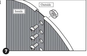
e. Cover the seam and bolt heads on the inside of the pool wall completely with 2" (50 mm) duct tape.
