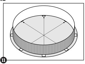
b. Adjusting the pool to the proper shape may cause the base rails and base plates to slip out of alignment a little. Recheck all of the base plates to make sure each one is centred where the base rails meet.
