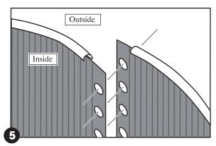
b. To line up the holes, make the circle bigger or smaller by nudging the base plates in or out with your foot.
