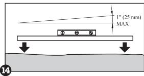
e. **Do not** fill in low areas. Filling will create an unsafe foundation for your pool. Small dips and hollows may be filled in, but the soil must be hardpacked with a tamping tool.
